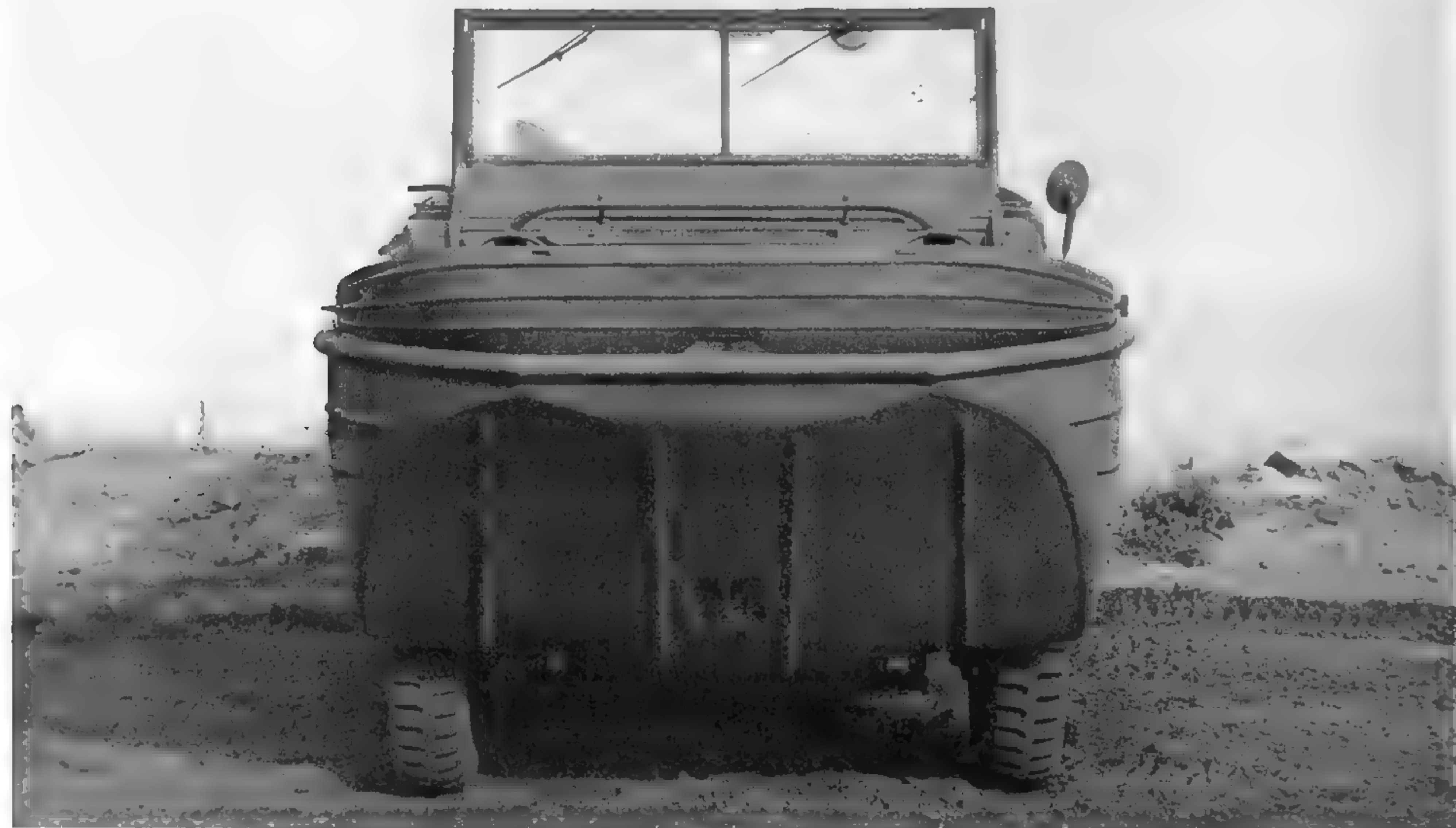
The hull of the GPA and DUKW were designed by the same firm. In this shot the surf shield has been placed in operating position, and the engine-cooling door can just be seen beyond it in the open position. (U.S. Army photo)
